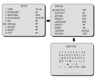
When adjusting the noise reduction level in the NR mode, remember that the higher the level set, the more the noise level will be reduced, as will the brightness of the image.
